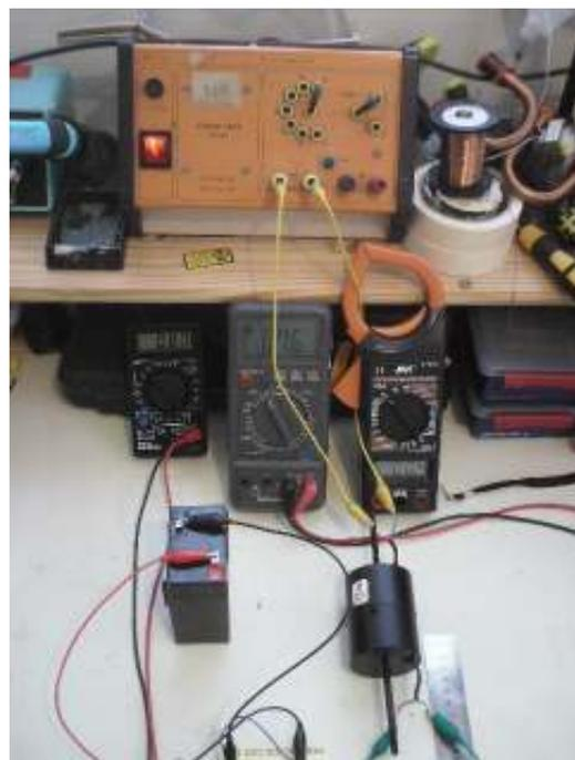
Coils close together – charging a 6v battery
