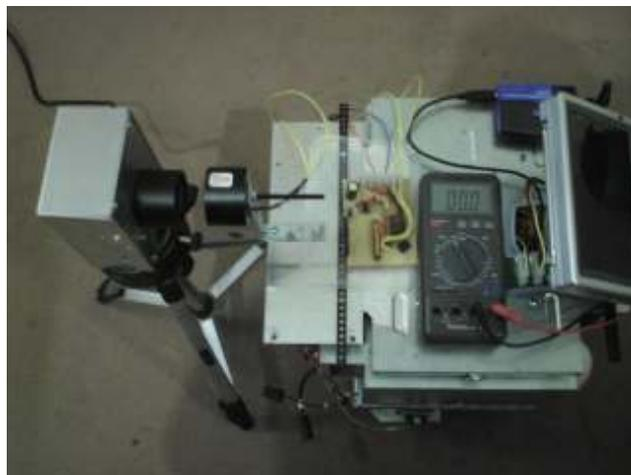
The robot and the wireless charger with a multimeter. Note that the reading is 0v because the coils are apart.
