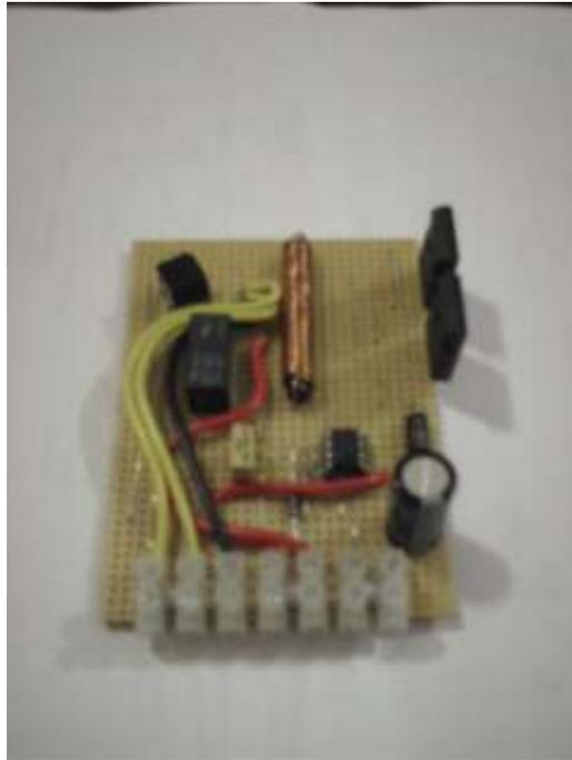
I have opted to charge the batteries in my robot at a rate of about 0.1C. The charge rate or C as it is known, is a percentage of the nominal current capacity of a battery. In the case of the 914, there are two 9Ah batteries connected in parallel inside it, providing 18Ah of service therefore for this configuration 1C is 18.
