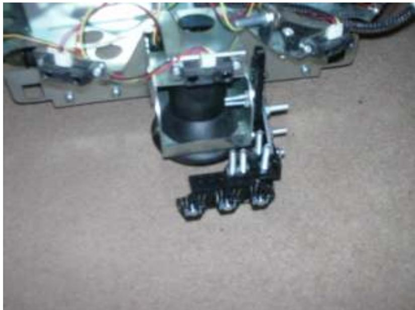
I located the sensors on the front castor wheel and just above the floor so reflections would be minimal.
