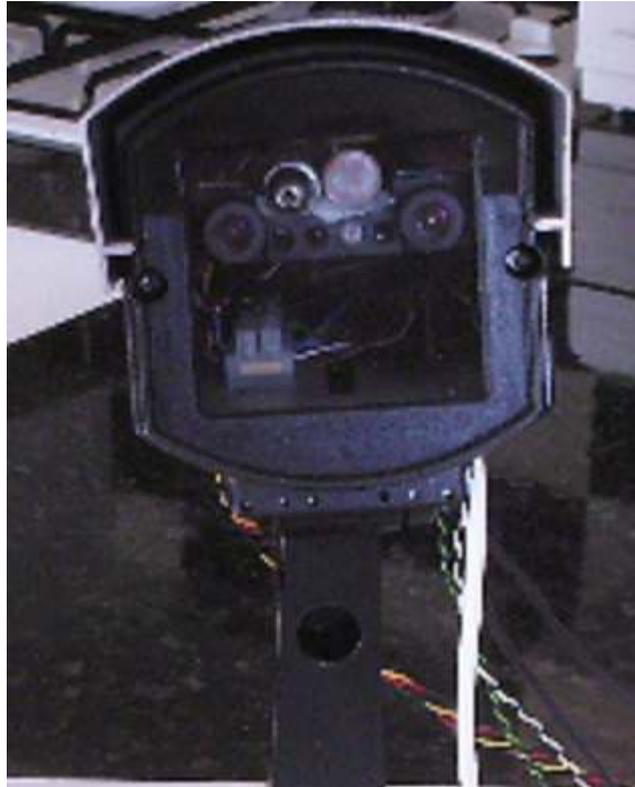
Its got the two cameras, a light sensor, laser and an infrared transceiver for decoding signals from a remote control.
