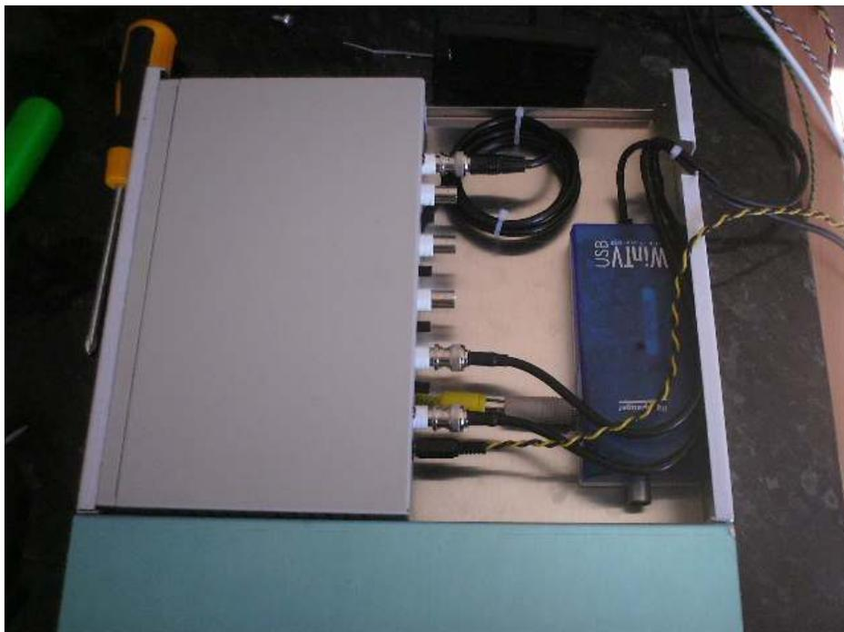
The nice thing is that the multiplexer and cameras use +12v which means you can power them easily from the 914 computer supply. I have capacity here for another two video cameras.
