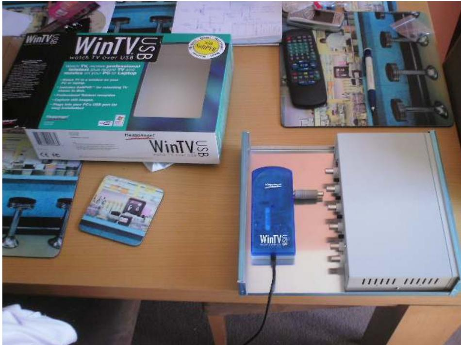
The computer tank on the 914 is too small to fit PCI cards into so the obvious choice of video input device would be an external USB device like the Hauppauge WinTV USB. I got an enclosure and wired it all up.
